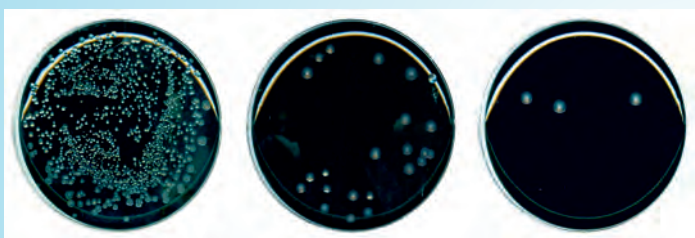
Obvious evidence in a petri dish: The growth of pathogens (pictured: legionella bacteria) can be evidently reduced due to antimicrobial additives.
