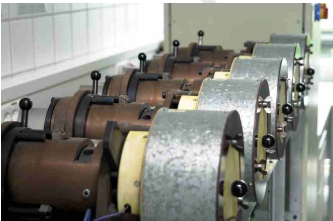
Diagram 2: FE9 test run with angular contact ball bearings 529689 (7206 B), mounting type A, i. e. open bearing; axial load F = 1,5 \text{ kN} ; speed n = 6000 \text{ min}^{-1} ; temperature +160 \text{ °C} Lubrication with THERMOPLEX® 2 TML
